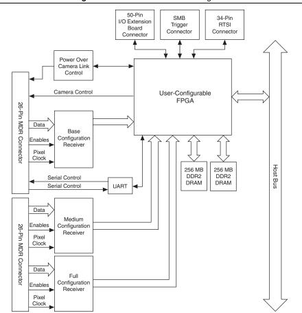
Figure 4. NI 1473R-LX110 Block Diagram
